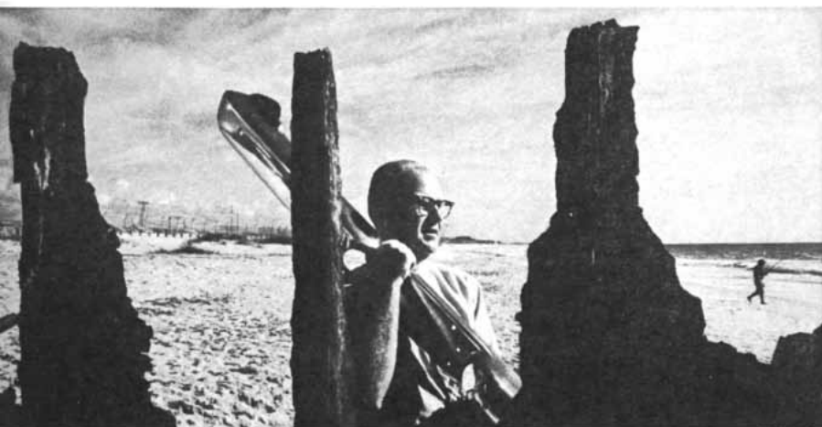
Vic holds a nickel-chrome plated automobile bumper which was tested in the corrosive seaside atmosphere.
