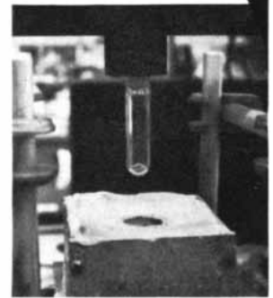
To prevent loss of mercury as vapor, all operations are at room temperature until oven is raised around tube containing pad, which then releases Hg vapor for atomic absorption photometry at 2537A.
