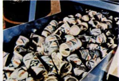
Used cans pass through a magnetic separator and are then shredded.
