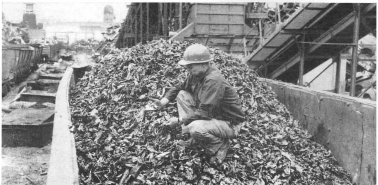
SHREDDING TECHNIQUE was recently developed for turning worn-out or wrecked automobiles into scrap that can be recycled
