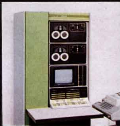
PDP-12, the total computer system with built-in graphic display, built-in operator/machine interaction, built-in analog capability. Primarily for the laboratory but finding wide applications in industrial control and education.
