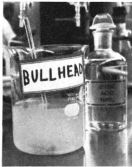
Homogenized fish marinated in \text{HNO}_3 to keep mercury in solution as \text{Hg}^{++} .
