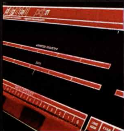
PDP-11: DIGITAL's new 16-bit computer with the modular approach, featuring UNIBUS™, an entirely new computer concept. Configurations include several for the OEM that sell for less than $5,000 in quantity, plus complete general purpose machines and software for the end-user.
