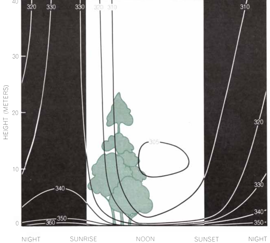
VERTICAL DISTRIBUTION OF CARBON DIOXIDE in the air around a forest varies with time of day. At night, when photosynthesis is shut off, respiration from the soil can raise the carbon dioxide at ground level to as much as 400 parts per million (ppm). By noon, owing to photosynthetic uptake, the concentration at treetop level can drop to 305 ppm.
